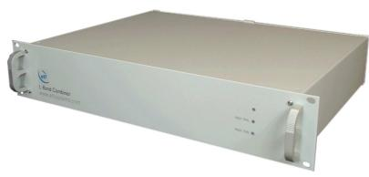
This single 16-way active Combiner operates over the L-band frequency range of 850-2150MHz. It is housed in a 2U high chassis and benefits from dual redundant power supplies for reliability in service.
